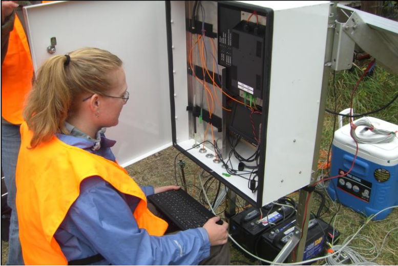
Jevon Harding (MS Hydro '12) using a distributed temperature sensing system at a tributary of the East Fork of the Jemez River.
