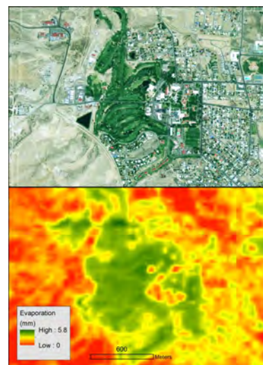
Michael Wine's (Ph.D. Hydro) project uses satellite imagery to map consumptive water use (evapotranspiration) on Tech's campus.
