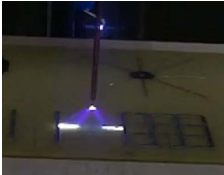
Figure 78 - Example of surface flashover seen in Pattern 1
