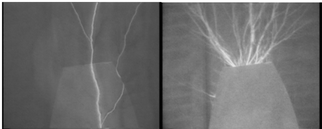
Figure 18 - UV spectral image of blade with round receptor on one side (Left – negative polarity; Right – Positive polarity) (Hernández et. al., 2010)
