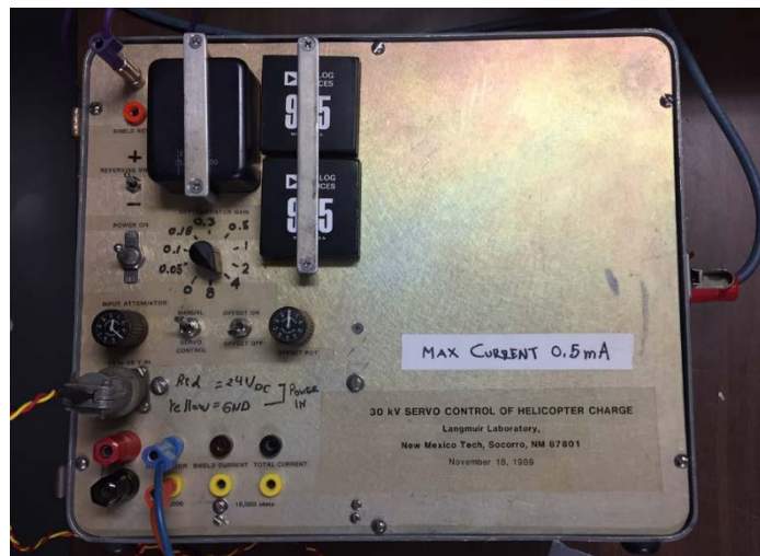
Figure 57 - 30 kV DC Power supply
