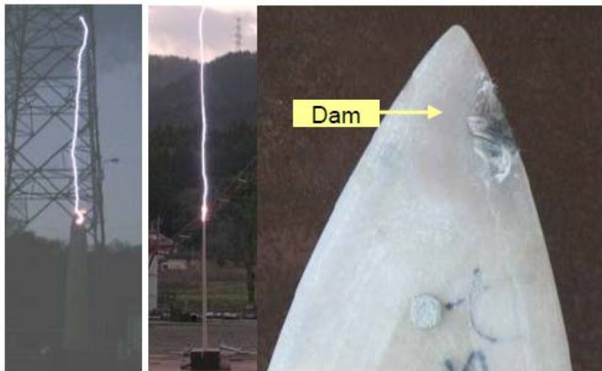
Figure 10 - Lightning attachment in Blade with receptor; Modified from (Yokoyama et al., 2014)
