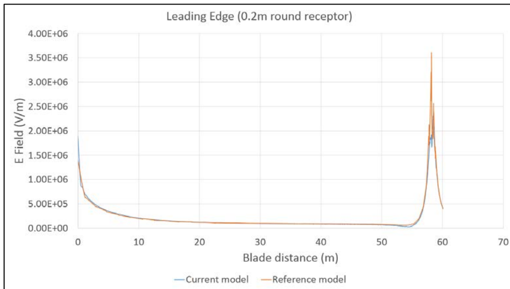
Figure 47 - Comparison of electric field along leading edge of reference and current model (0.2 m round receptor)
