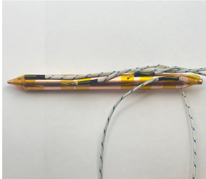
Figure 4.2: Thermocouples Taped on with Thermal Tape
