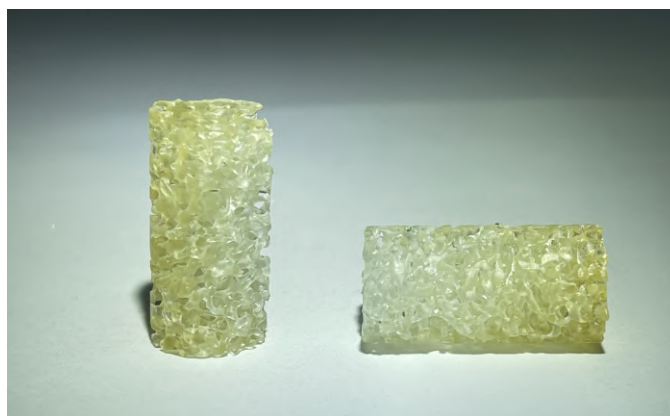
Figure 3.12: Two Successful Prints to the Correct Diameter. Left: Printed Vertically Right: Printed Horizontally
