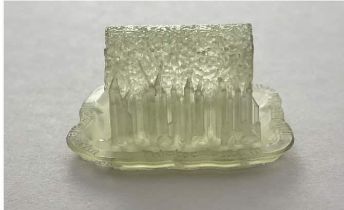
Figure 3.11: Failed Test Print. It Can be Seen That the Resin is Cured Inside of the Structure, Making it Solid.
