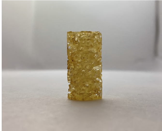
Figure 3.14: Biomimetic Structure After Integrity Test
