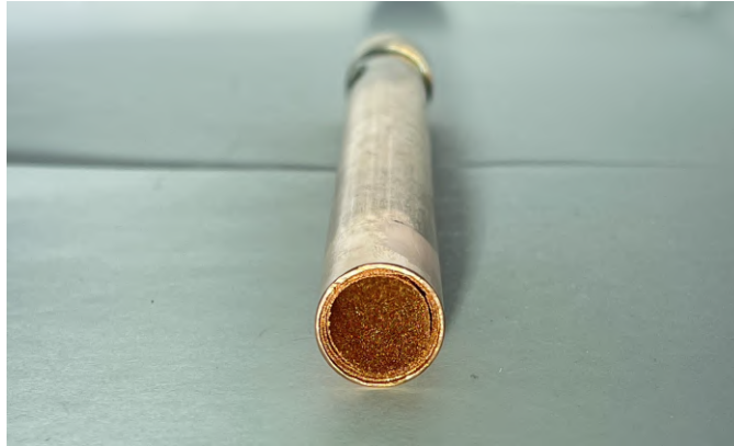
Figure 3.7: Traditional Heat Pipe with the Wick Inserted
