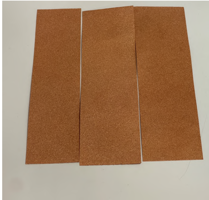
Figure 3.6: Cut Copper Foam
