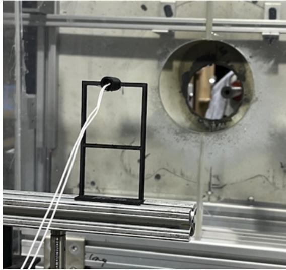
Figure 4.3: 3D-printed Onyx detonator holder with the detonator positioned squarely in front of the gun.
