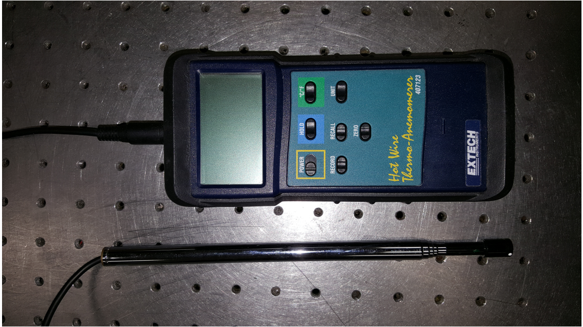
Figure 1.2: An example of a hot wire anemometer model number 407123 by EX-ETECH Instruments.
