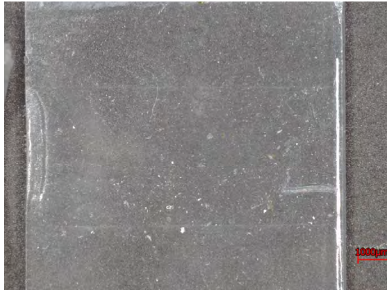
Figure 4.12: Test 38 flat substrate due to a failure to propagate across the gap.
