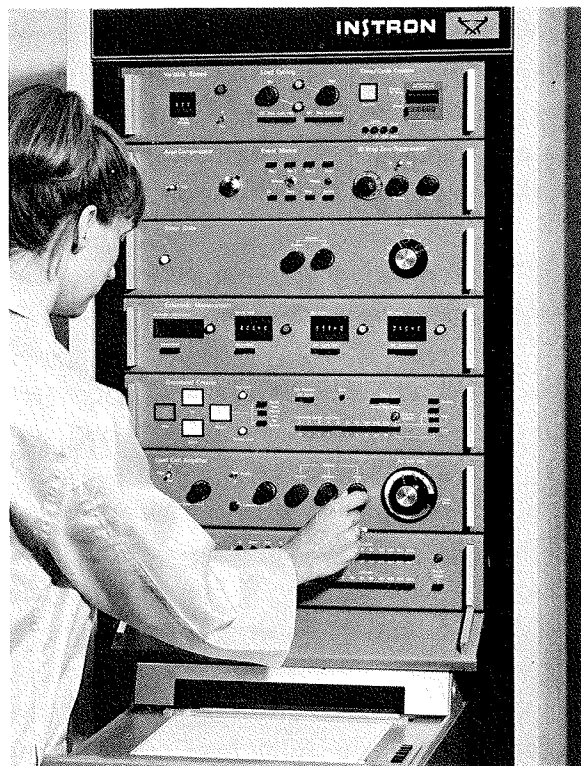
Figure 6-2. Balancing the Load Weighing System
