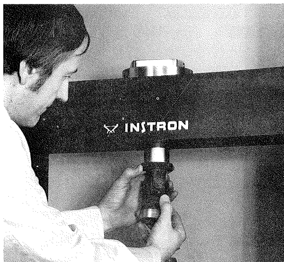
Figure 5-11. Attaching a Self-Aligning Coupling to a Tension Load Cell
