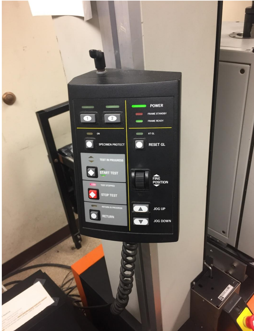
Instron Control Panel with “Jog Up” /“Jog Down” buttons and a “Fine Position” knob.
