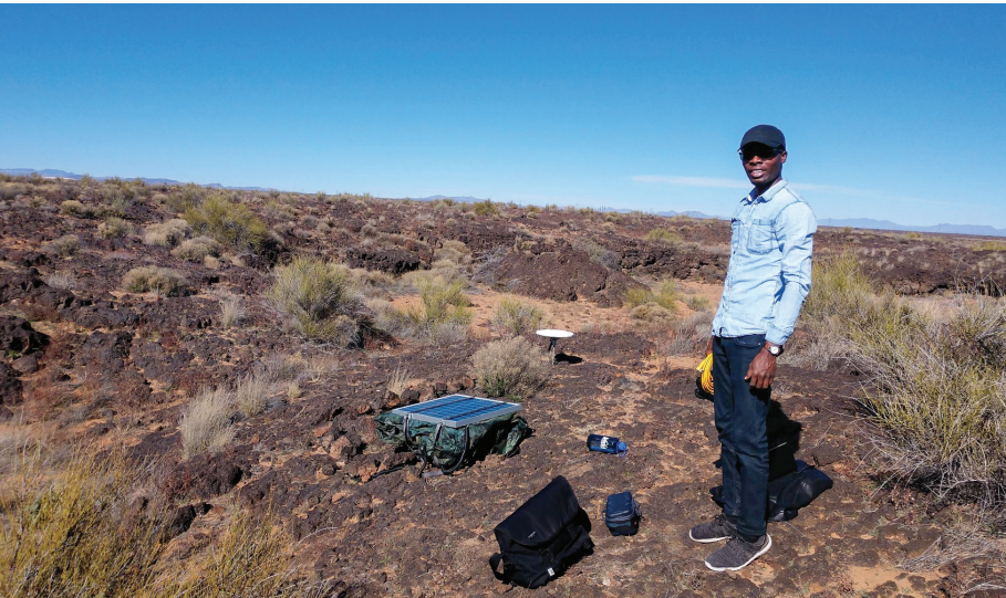
A graduate student maintaining a GPS station monitoring groundwater in southern New Mexico
