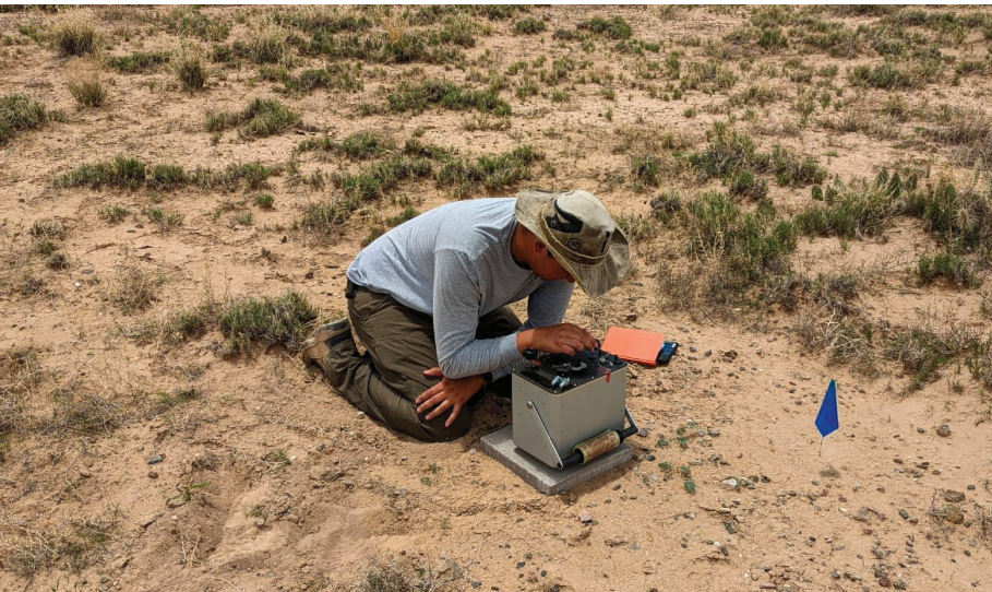
An undergraduate running a regional gravity survey on Sevilleta National Wilderness Refuge
