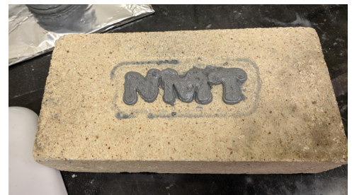
A sample of rocket propellant printed by NMT students
